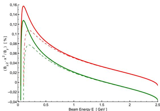
Figure 2: Sextupole field component [%] at  $r = 20$  mm during energy ramping, due to eddy current only (red curves) and overall component (green curves) with an energy ramping from 0.05 (solid curves) and 0.1 GeV (dotted curves) to 2.5 GeV.
