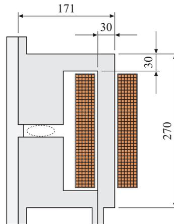
Figure 6: Horizontal Steerer Cross Section
