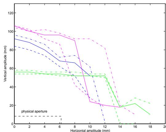
Figure 3: Dynamic aperture at 2.5 GeV for the low emittance optics for different sextupole components and energy spreads.
