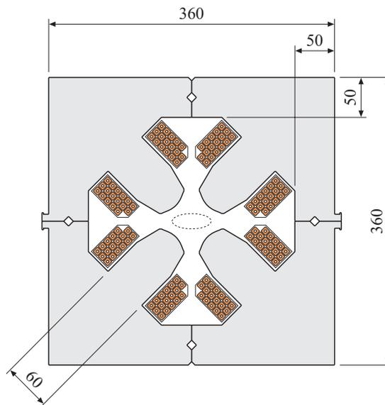
Figure 4: Quadrupole Cross Section
