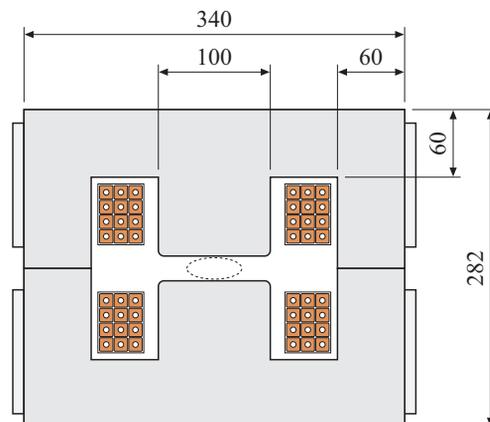
Figure 1: Dipole Cross Section
