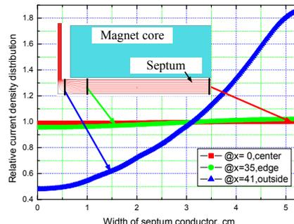
Figure 6: Current distribution in septum conductor
