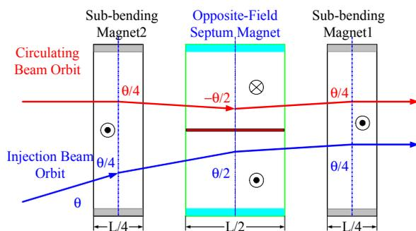
Figure 1: Principle of opposite-field septum magnet.
