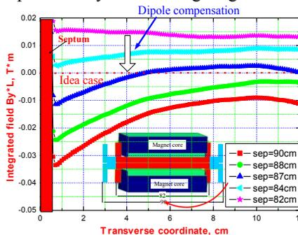
Figure 8:  $B_y \cdot L$  with respect to the septum length
