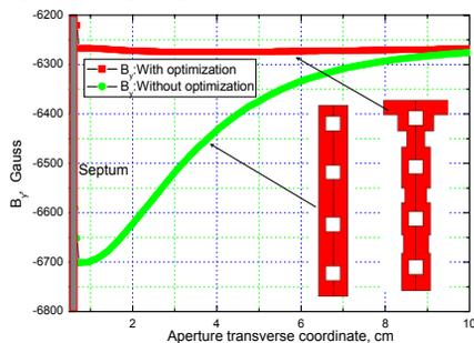
Figure 4: Septum conductor shape optimization
