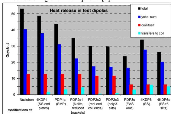
Figure 2: Loss reduction during R&D phase for the triangular cycle 1Hz, 2T.
