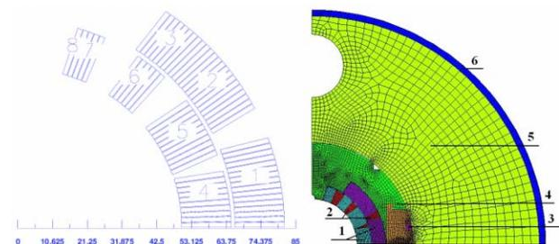
Figure 3: 2D coil design (left) and FEM model for mechanical analysis of SIS300 dipole (right). 1-coil, 2-inter-turn spacers (wedges), 3-key, 4-collars, 5-yoke, 6-outer cylinder.
