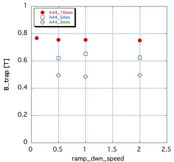
Figure 5: Trapped field as a function of the normalized ramp-down speed for different samples.
