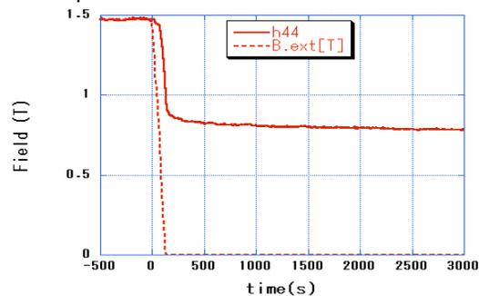
Figure 2: Trapped field by the Hall probe located at the position  $(i,j)=(4,4)$  where  $i$  and  $j$  run from 1 to 6, respectively, as indicated in Fig.1.
