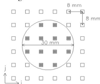
Figure 1: Top view of Hall array.
