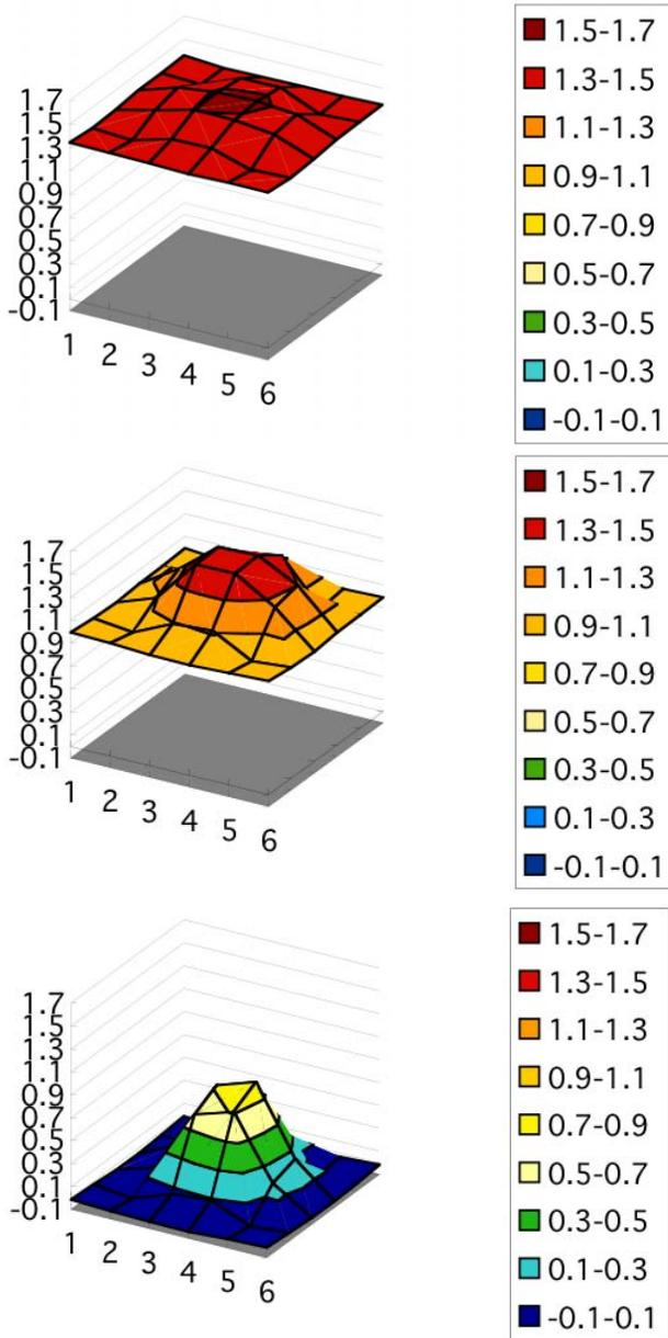
Figure 3: Field distribution at  $t=20$  s, 50 s and 800 s when the initial external field is 1.5 T, from top to bottom.
