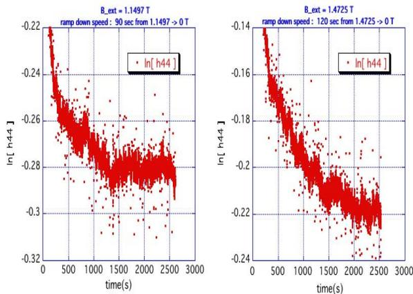
Figure 6:  $\text{Log}(B_{trap})$  vs. time when  $B_{init} = 1.15$  T (left) and 1.5 T (right) monitored by the Hall probe located at the position  $(i,j)=(4,4)$  near the center of the sample.
