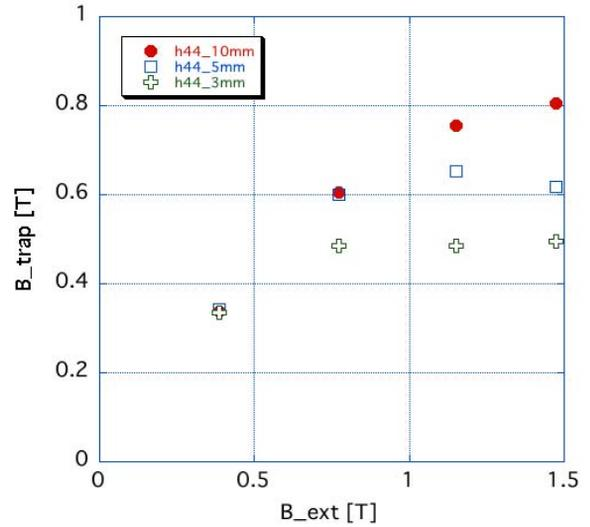
Figure 4: The trapped field monitored by the probe near the center of the sample is plotted against the initial external field.
