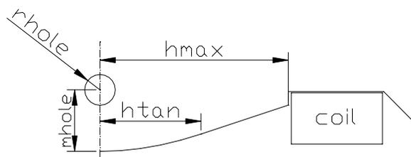
Figure 1: Parametrized pole shape with a protruding coil.
