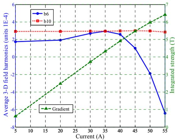
Figure 4: Quadrupole integrated field results (at 30 mm reference radius).
