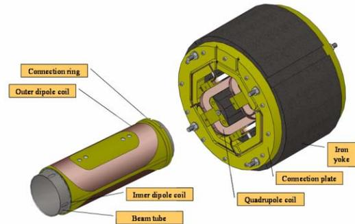
Figure 5: Dipoles and quadrupole coils assembly.
