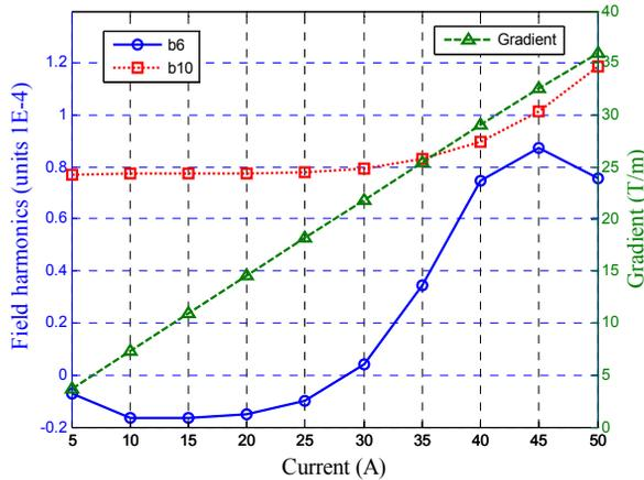
Figure 2: 2D quadrupole field optimization results (at 30 mm reference radius).
