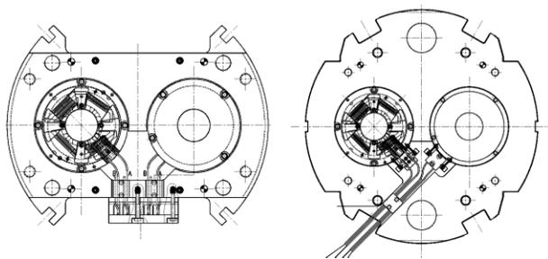
Figure 1: Cross-section of MQTLI- and MQTLH- assemblies
