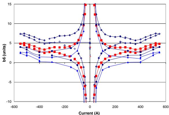
Figure 4: Normal dodecapole as a function of current.
