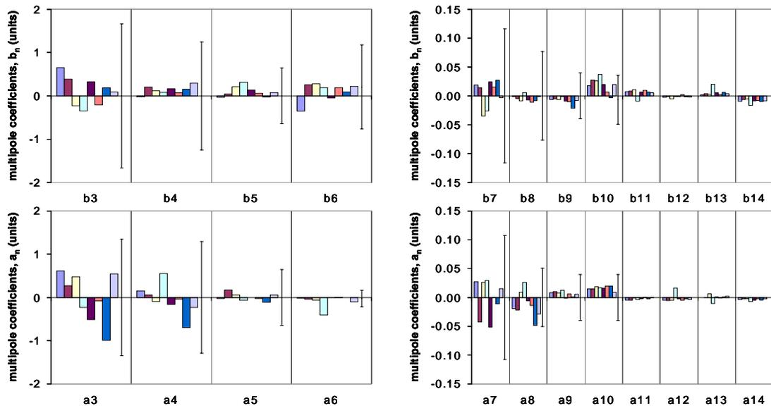
Figure 2: Measured multiple components of the LQXB quadrupoles at collision energy in units of  $10^{-4}$  at  $R_{ref}$  of 17 mm, compared with target values (error bars).
