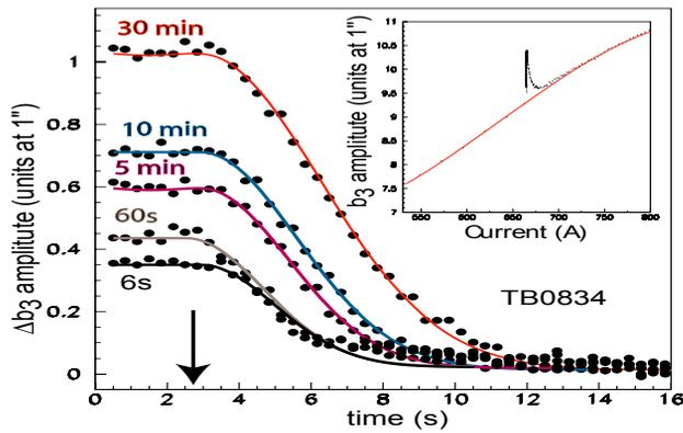
Figure 2: Typical sextupole decay amplitudes  $\Delta b_3$  versus the snapback time for magnet TB0834. The different fits with corresponding points are the measured snapbacks for different IP durations. The arrow points at the beginning of the snapbacks. The inset shows the correction to the  $b_3$  hysteresis loop, which was done by a second order polynomial.
