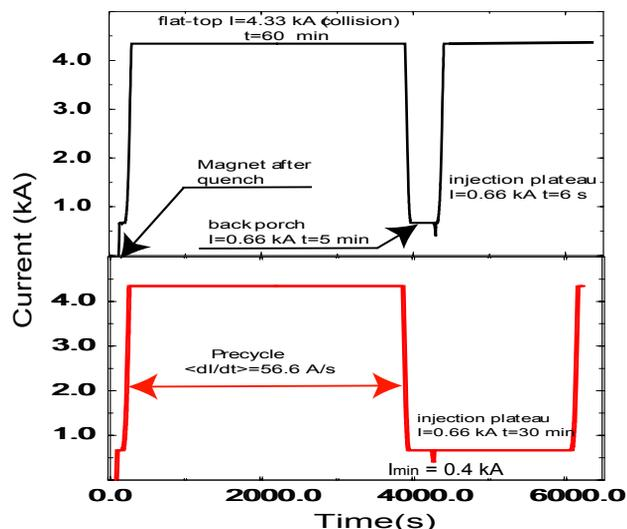
Figure 1: Two typical current cycles used in the decay and snap-back measurements. The upper (lower) plot represents a cycle with the shortest (longest) IP duration of 6 s (30 min).
