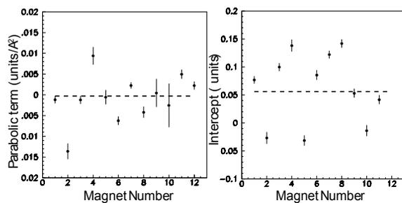
Figure 4: The parabolic term returned by the fit of  $\Delta b_3^{dec}$  versus  $\Delta I$  distributions for the set of 12 Tevatron dipoles (right). The same plot but for the intercept in case of the linear fit is shown on the right. The dashed lines represent the average values.
