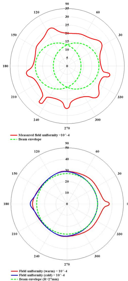
Figure 5: Dynamic apertures of the present single-aperture NbTi LHC IR quads (top) and 2-in-1 Nb<sub>3</sub>Sn quads (bottom).
