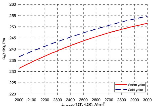
Figure 3: Quench gradient at 1.9 K.
