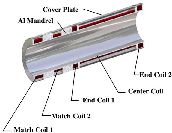
Figure 1: The Tracker Magnet Cold Mass Assembly
