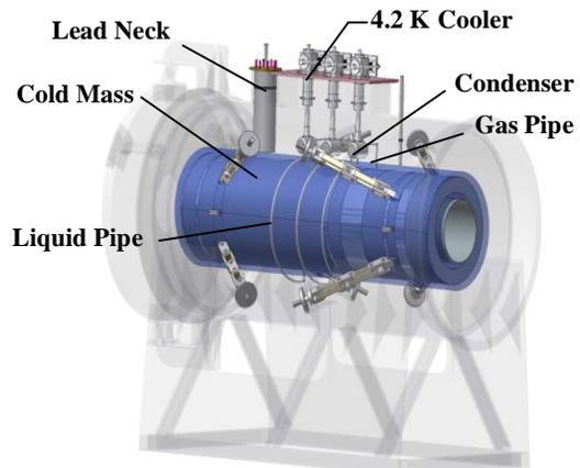
Figure 2: Magnet Cold Mass and Cryostat
