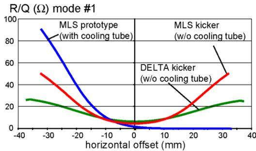
Figure 5: R/Q-factors of the first resonant mode in the MLS and DELTA kicker respectively computed at different horizontal offsets. Asymmetric fields can be induced by implementing a cooling tube.
