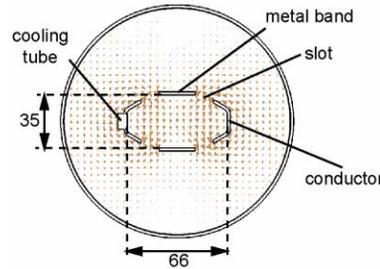
Figure 2: Cross-section of the MLS kicker model with the magnetic kicker field as simulated with MWS.
