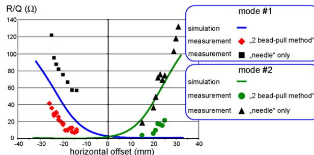
Figure 9: Measured R/Q-values of mode #1 ( $f_0 = 213.5$  MHz) and mode #2 ( $f_0 = 221.7$  MHz) respectively at different horizontal offsets. Simulated results are given for comparison.
