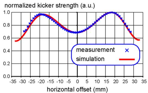
Figure 3: Measured and simulated magnetic kicker strength at different horizontal offsets.
