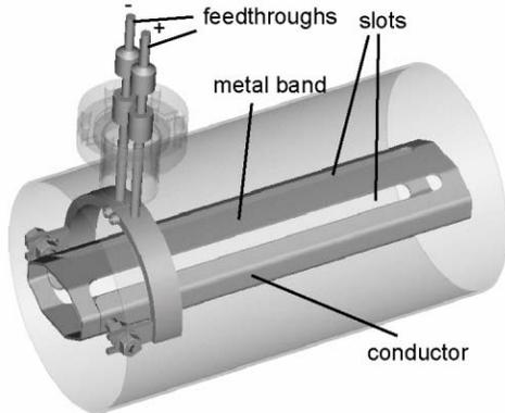
Figure 1: Transparent view of the MLS kicker showing the slotted pipe and electrodes inside the vacuum vessel.
