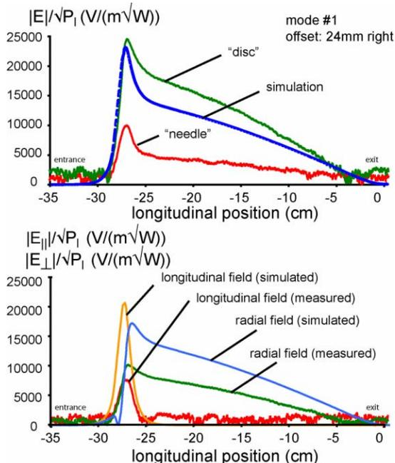
Figure 8: Measured and simulated fields  $|E|/\sqrt{P_1}$  of the first mode in the MLS kicker at a horizontal offset of 24 mm towards cooling tube. At the top the absolute field values are shown, whereas the purely longitudinal and radial fields are shown at the bottom.
