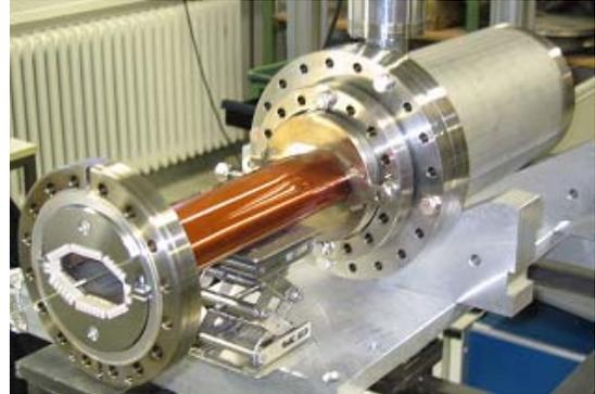
Figure 7: Setup showing the MLS kicker model with an additional vacuum chamber flanged on one side.
