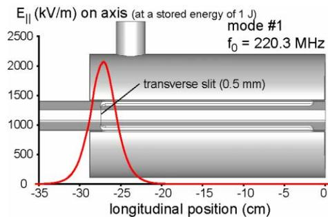
Figure 4: Computed on axis electric field of mode #1.
