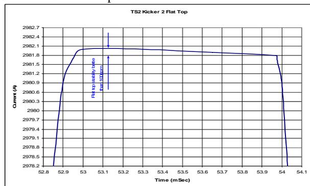
Figure 7: Simulated 10Hz pulse flat top.
