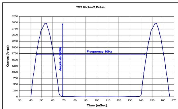
Figure 6: Simulated 10Hz pulse.
