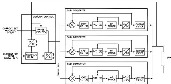
Figure 4: Septum Converter (one power cabinet).
