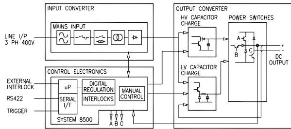
Figure 5: Danfysik 10Hz Pulsed Power Converter.
