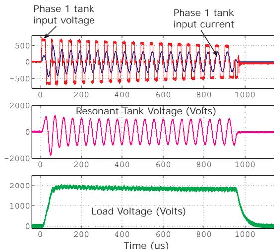
Figure 3: Waveforms measured during a 250kW output pulse.
