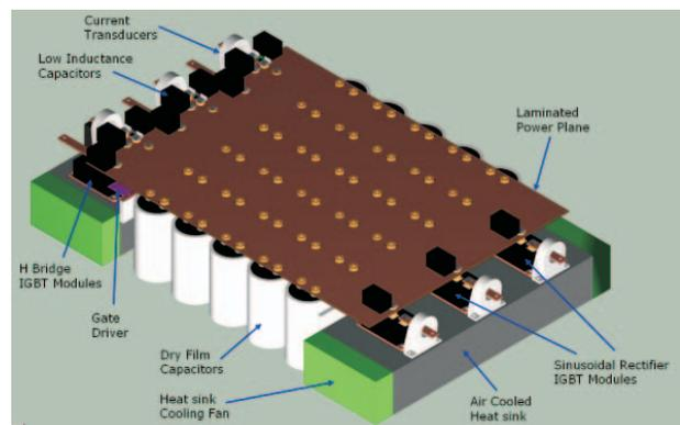
Figure 2: CAD model of power circuit showing Sinusoidal Rectifier, DC link, H-Bridges.
