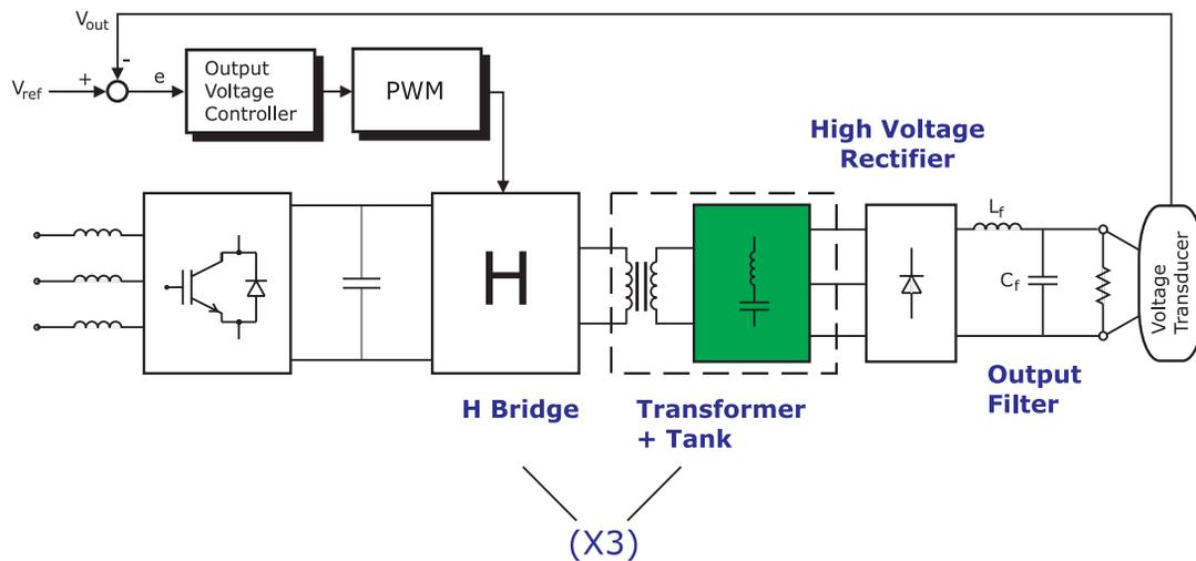
Figure 1: Block diagram of DC link based converter.
