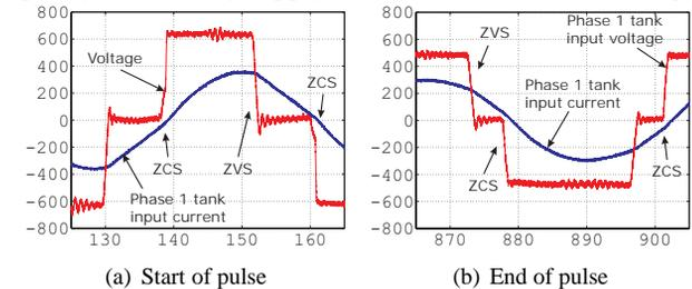
Figure 4: Waveform detail showing that soft switching is achieved for all IGBTs throughout the pulse.
