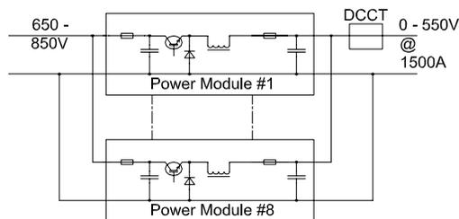
Figure 1: Dipole Converter Topology.
