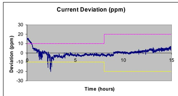
Figure 4: Q Converter Stability
