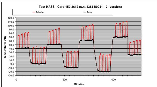
Figure 3: HASS component temperature stress profile
