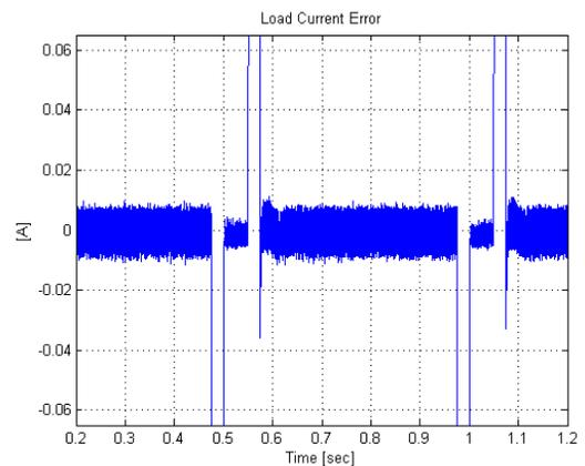
Figure 6: Load current error (zoom),  $V_{line}$  at 90%.
