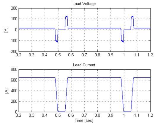
Figure 4: Load voltage and current  $V_{line}$  at 90%.
