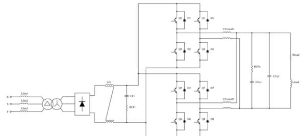
Figure 2: Topology of sextupole magnet power supply.
