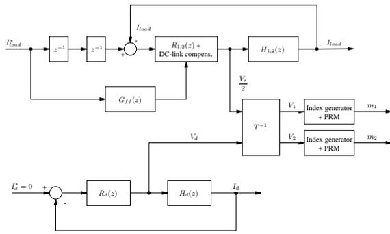
Figure 3: Structure of digital controller.
