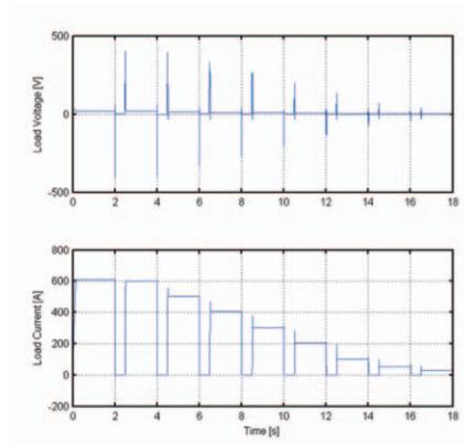
Figure 1: Load voltage and current during a treatment plan where the beam energy decrease cycle by cycle.
