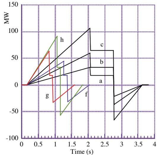
Figure 2: The active power of the MR (bending magnets and quadrupole magnets) for the various operation patterns. Parameters of each pattern are shown in Table 1.
