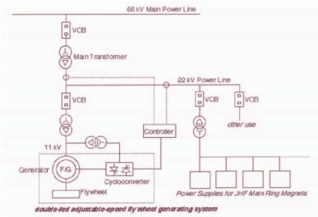
Figure 1: Conceptual block diagram of the power supply system with FWG for 50-GeV MR.
