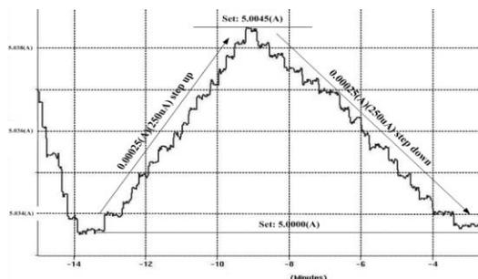
Figure 7: Output current step response of bipolar MPS.
