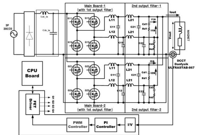
Figure 5: Circuit diagram of unipolar MPS.
