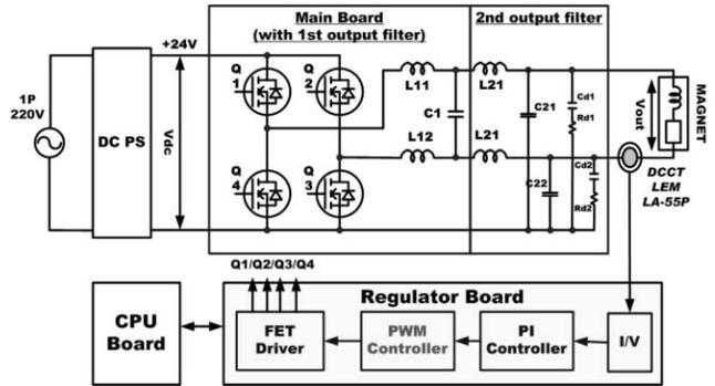
Figure 4: Circuit diagram of bipolar MPS.
