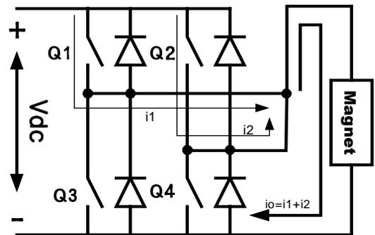
Figure 2: Unipolar MPS operation of full-bridge four-quadrant DC/DC converter.
