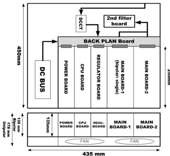
Figure 3: Configuration diagram of PAL Linac new MPS.
