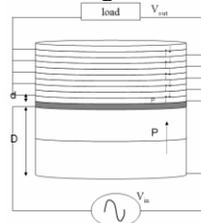
Figure 1: The prototype of the step down piezo transformer.
