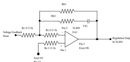
Figure 7: Circuit diagram for voltage feedback control loop.
