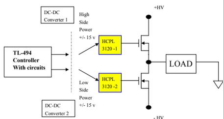
Figure 6: Half bridge driver and topology.
