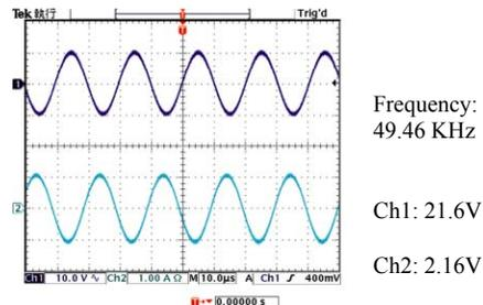
Figure 2: The resonant frequency-testing diagram of the step down piezo transformer.
