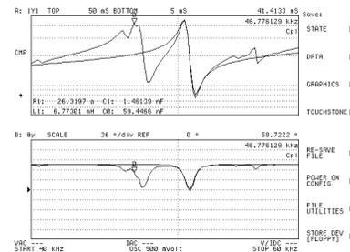
Figure 5: Impedance response diagram of the secondary characteristic for the step down piezo transformer.
