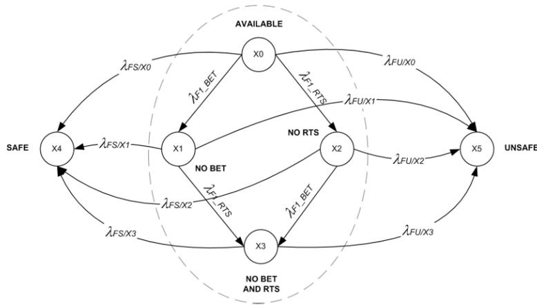
Figure 2: The state transition diagram of the LBDS failure processes.
