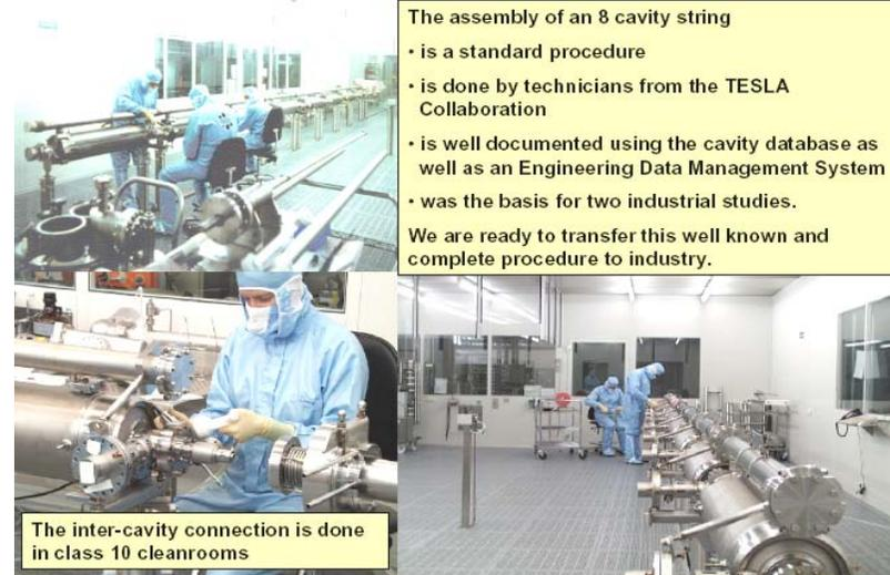
The inter-cavity connection is done in class 10 cleanrooms
