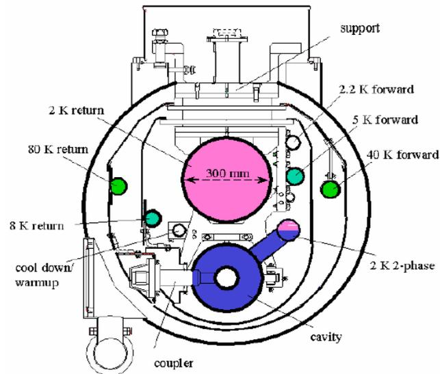
Figure 3.3.2: Cross section of cryomodule.
