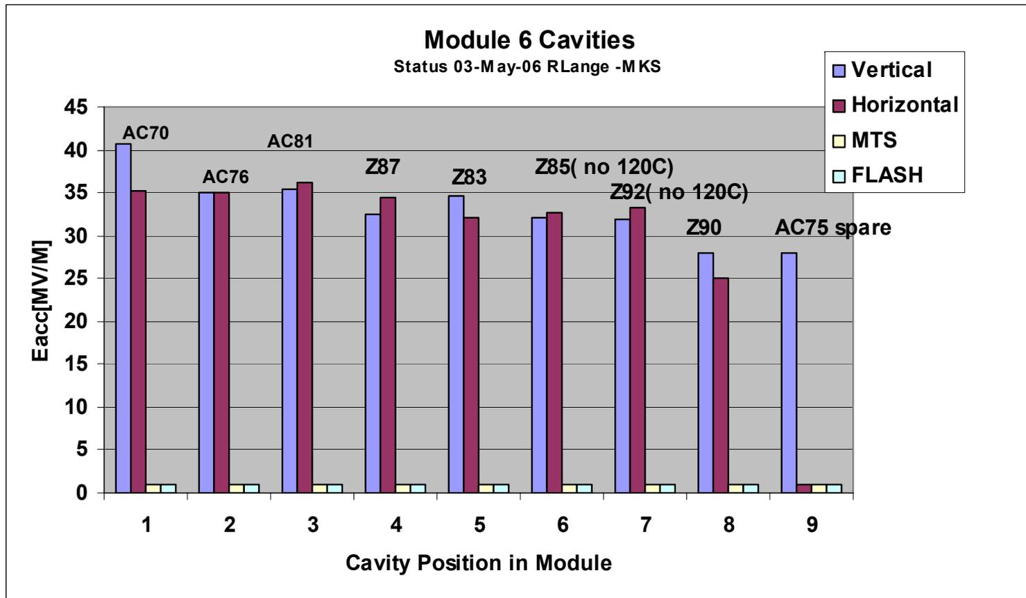
**ITRP R1 issue (2004) : The feasibility demonstration of the TESLA energy upgrade to about 800GeV requires that a cryomodule be assembled and test at the design gradient of 35MV/m.**
