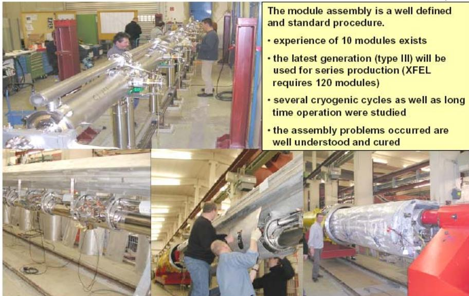
The module assembly is a well defined and standard procedure.
