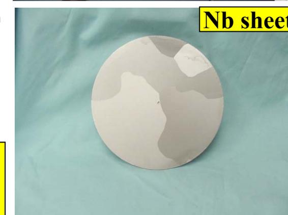
**Large grain Nb sheet production can bring a cost down.
