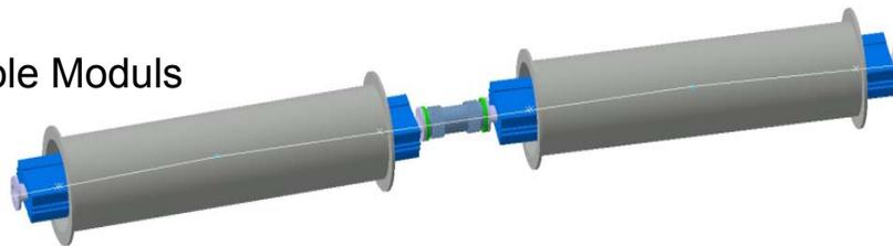
Quadrupol unit of the arcs includes sextupole, BPM and collimator
