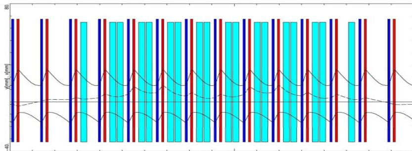
Optional for compression, fast extraction and shift of transition energy – almost dispersion free, good collimation
