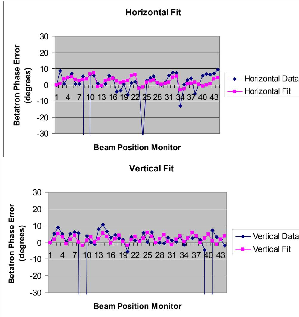
Plots show measured betatron phase error vs. model-based fit
