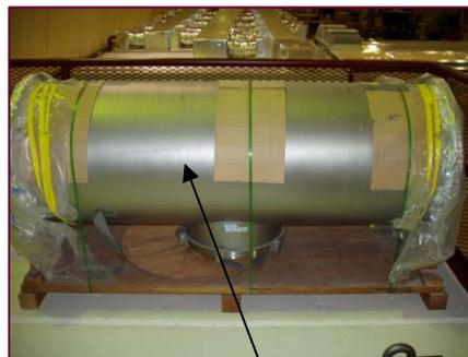
Stanford cryomodule and cavities at Daresbury
