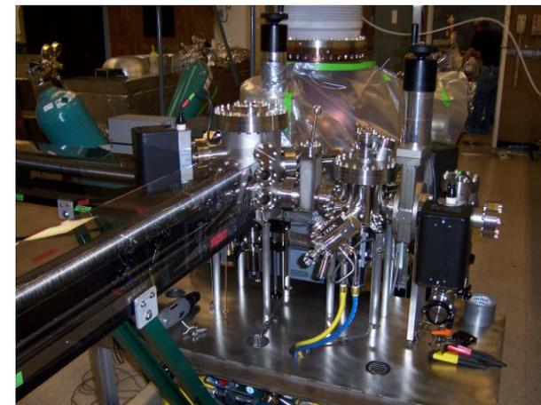
The photocathode load lock and preparation system, with translation mechanisms
