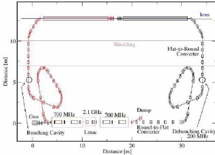
**RHIC electron cooler is based on a 200 mA, 55 MeV ERL
