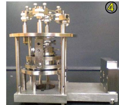
Photocathode Test Bench (Cathode holder)
