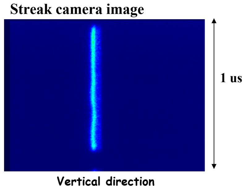
**The tail part of the bunch train is oscillating vertically.**
