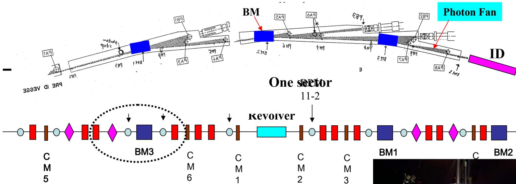
2. A fixed gap photon mask with a vertical aperture of 8 mm was installed in front of the Revolver, but no appreciable change.
