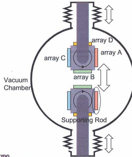
Permanent magnet structure is a revolving type with four arrays, which provides 4 different undulator periods of 10, 15, 20, and 24 mm.
