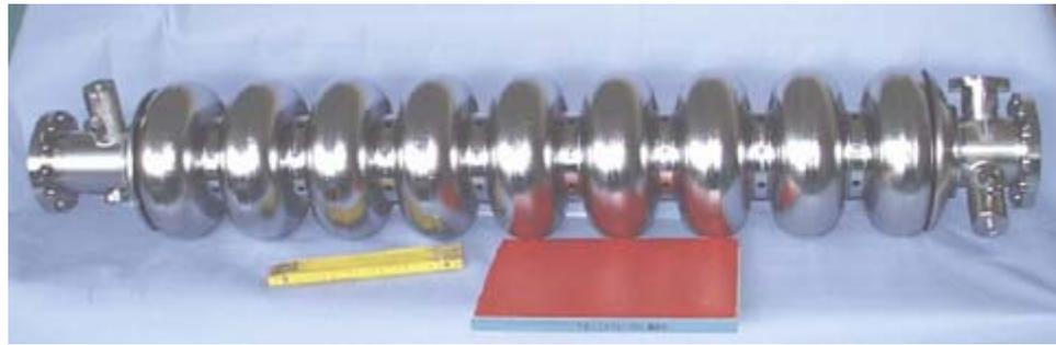
One standard **9-cell TESLA accelerating structure** operated as a  $\pi$ -mode standing-wave cavity.
