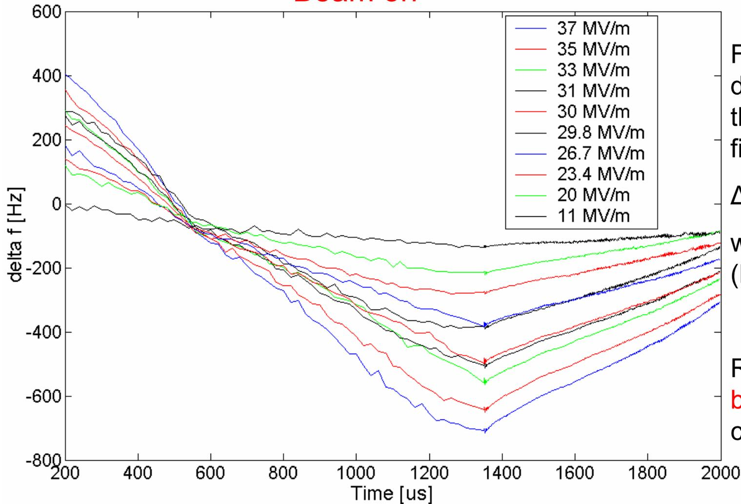
Frequency detuning due Lorentz forces of the electromagnetic field in the cavities:
