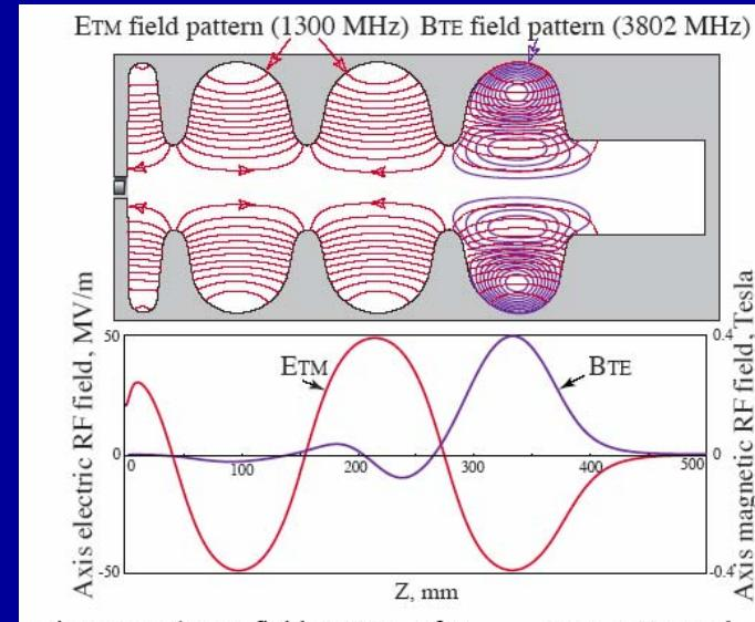
Figure 2: a) RF field pattern of  $E_{TM010}$  1300 MHz and  $B_{TE021}$  3802 MHz. b) Axis fields of the RF modes.(Color picture)
