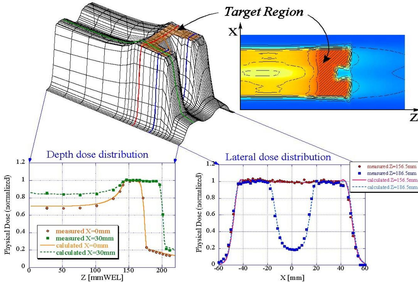
**Experiment of spot scan for irregular shape target**
