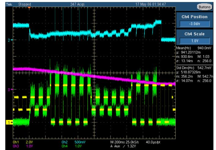
The spot scanning and layer stacking methods require an intensity modulation. Therefore, we have studied the dynamically intensity control. This figure shows three intensity steps during 50 ms. This figure shows sinusoidal intensity wave.
