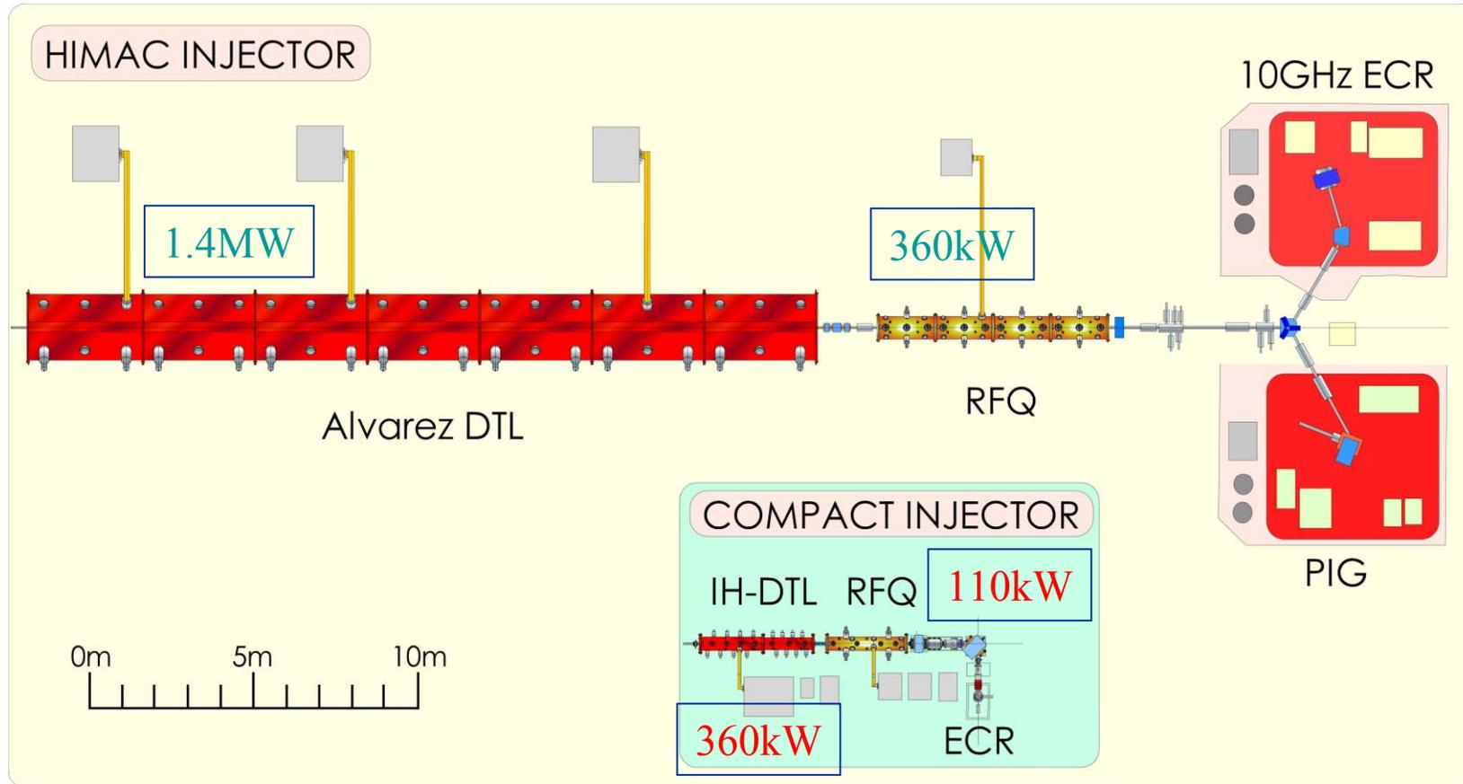
The injector linac cascade consists of RFQ and APH-IH linac. The RFQ accelerates  $C^{4+}$  ions from 10 to 600 keV/n. The APF-IH accelerates them to 4 MeV/n. Both the operation frequencies are 200 MHz.
