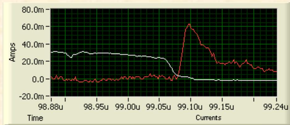
BCM signal (white) and photodiode signal (red). Observed dip was around 20%
