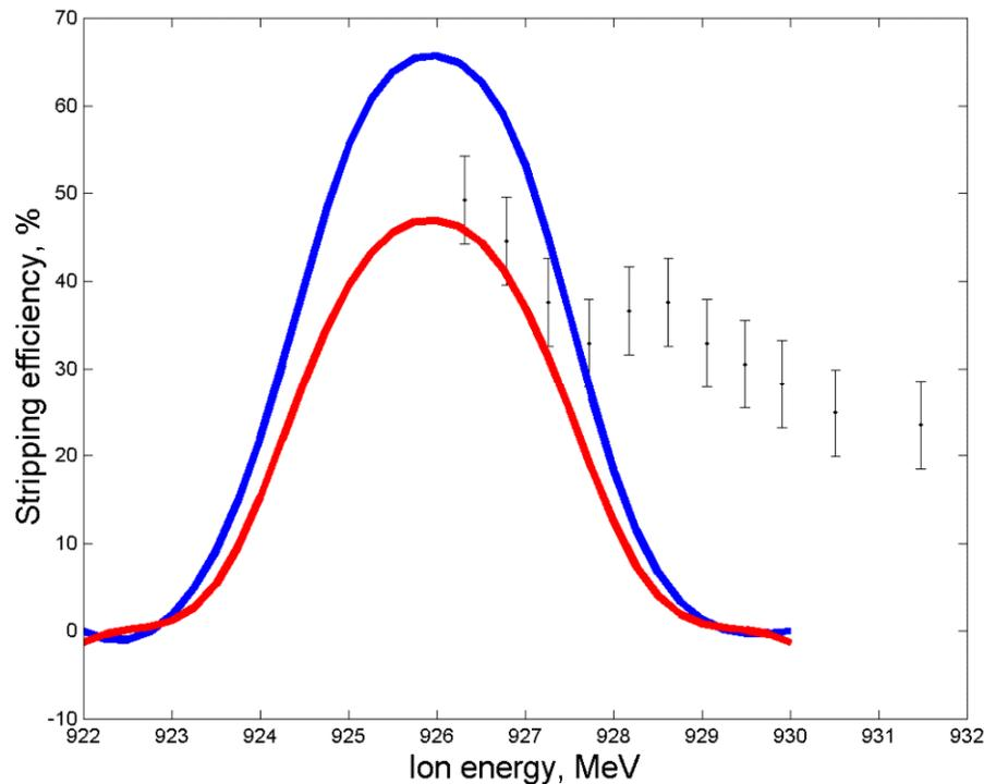
**Experimental data (dots with error bars) and two calculated efficiency vs energy curves for 0.8 mm (blue line) and 1.2 mm (red line) vertical sizes of the ion beam. Ion beam energy spread was 0.5 MeV in calculations. It seems that it was larger (see the experimental width is 2.5 larger).**
