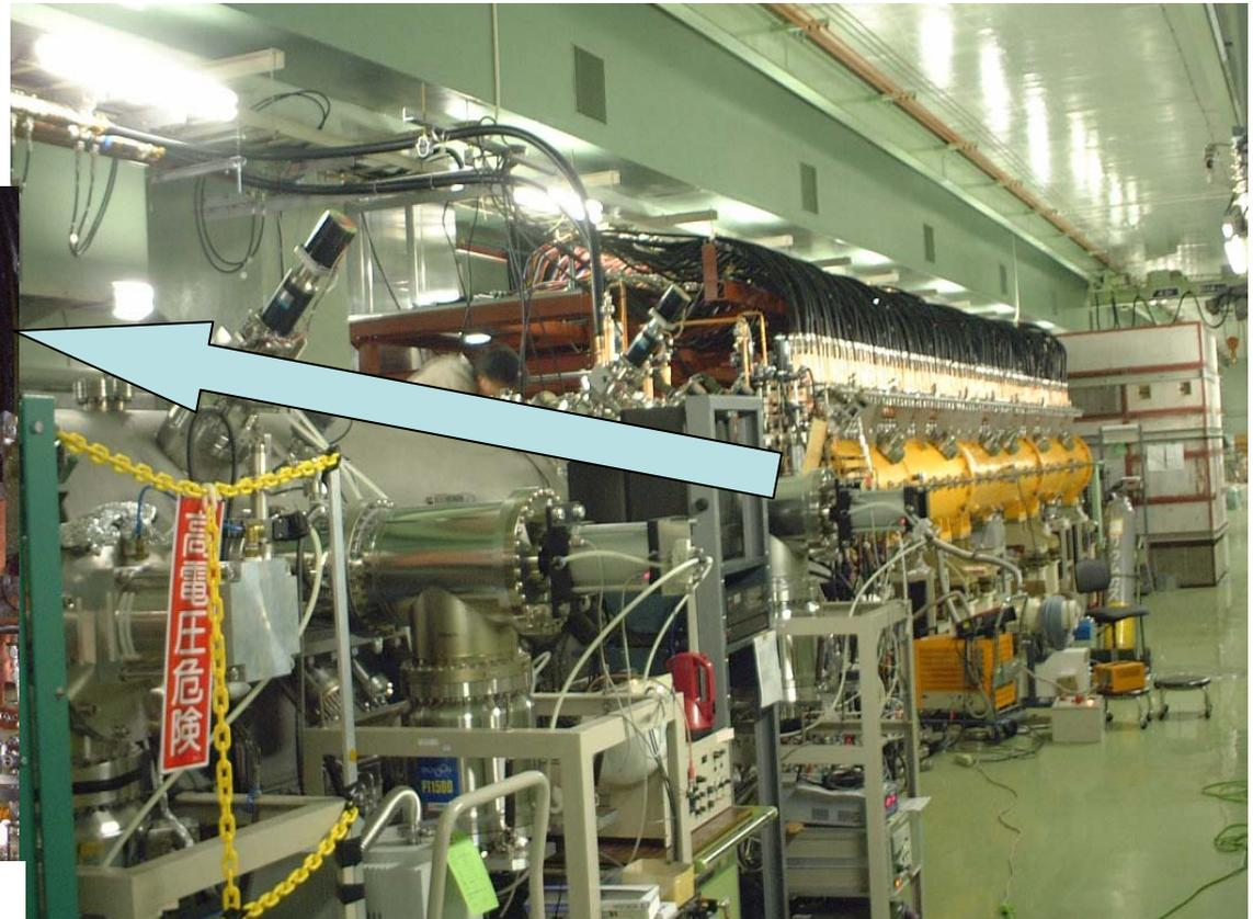
Photograph of the RFQ and DTL-1 (orange cavity).
