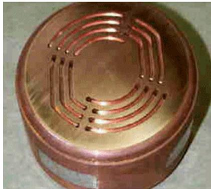
Grooves and through holes for water channel
