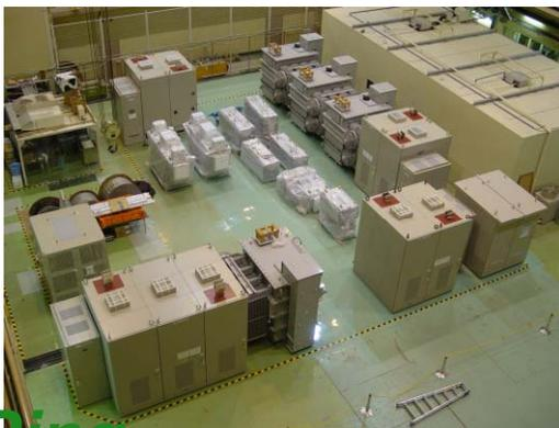
**Pulsed Bending Magnet for swinging the beams to MLF and MR**
