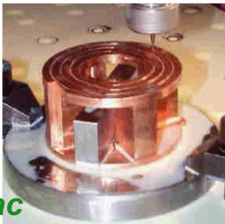
Forming the coil by wire cutting.
