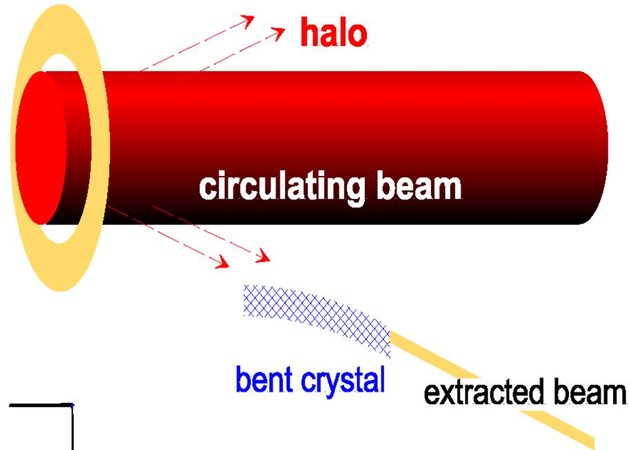
Channeling, scattering, and accelerator dynamics are essential in multi-turn, multi-pass process of crystal extraction (and collimation)
