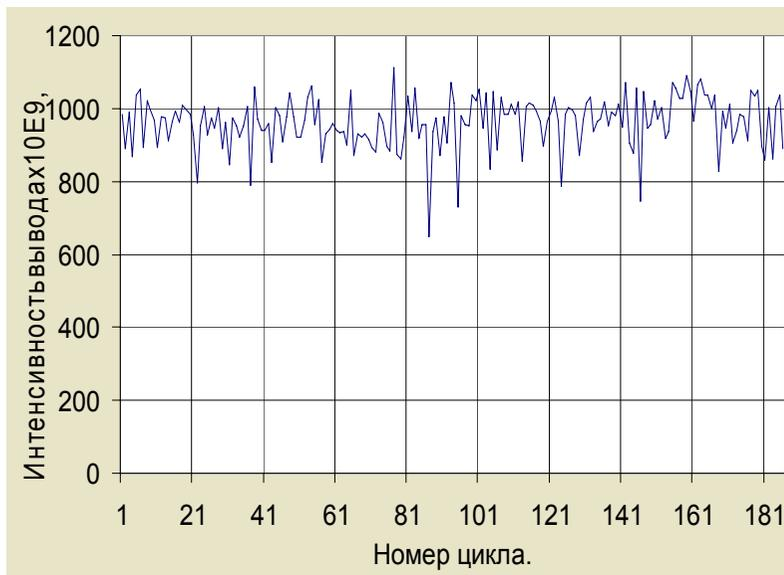
**Extracted beam intensity per cycle**
