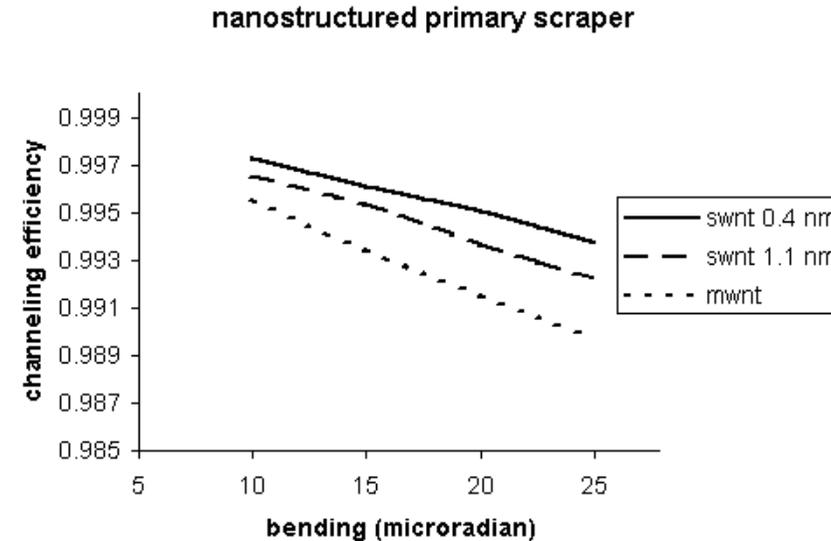
Nanostructured channeling material could be used for primary scraper
