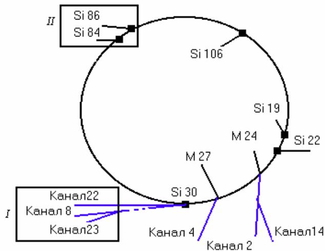
**Crystal systems extract 70 GeV protons from IHEP main ring with efficiency of 85% at intensity of  $10^{12}$ . Today, six locations on the IHEP 70-GeV main ring are equipped by crystal extraction systems, serving mostly for routine applications rather than for research**
