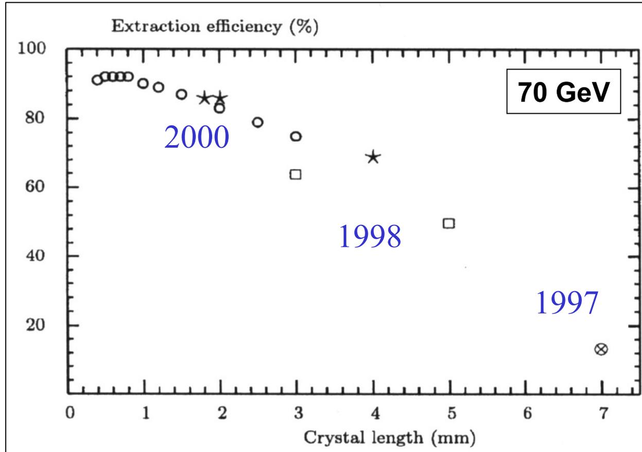
Measured efficiency of 85 % for 2 mm long crystals (highest ever)
