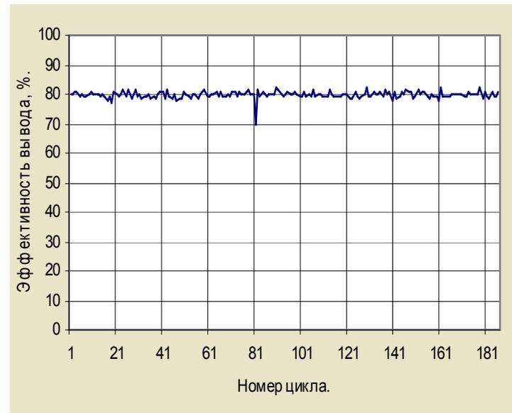
**Extraction efficiency measured by cycle**
