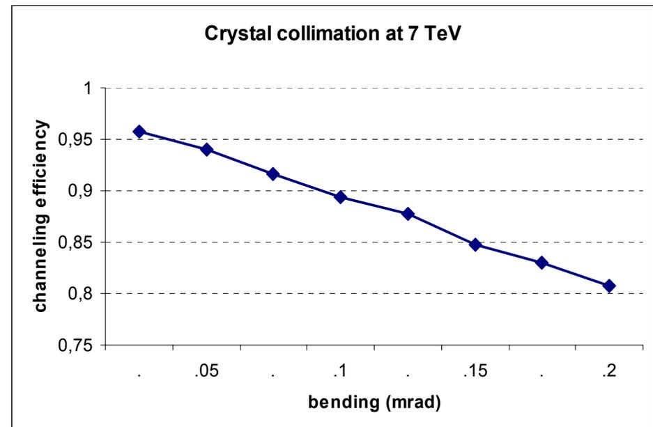
Channeling efficiency as a function of the crystal orientation angle. The orientation curve has  $\text{FWHM} = 7 \mu\text{rad}$  at top energy.
