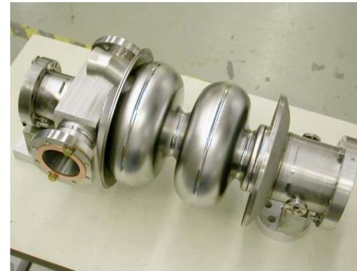
Injector: 5 cavities needed for ERL injector; prototype reached 21 MV/m; at 15 MV/m,  $Q \sim 10^{10}$
