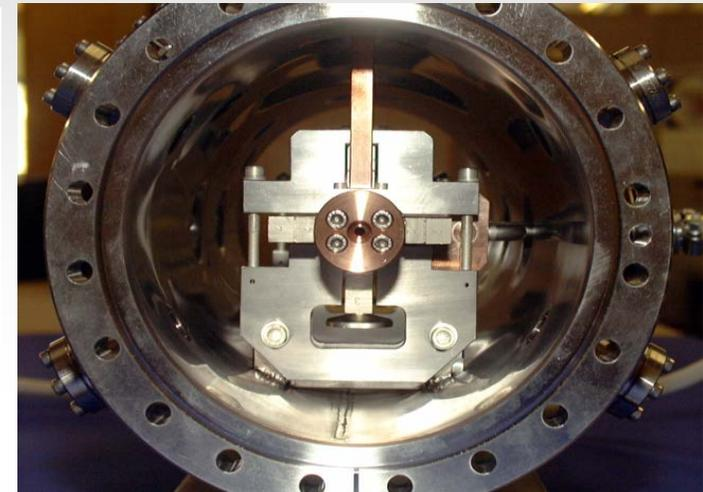
Test structure in external vacuum with clamped coupler cell
