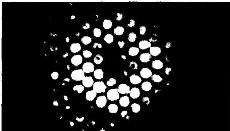
Fig.6. Picture of the neon-filled lamps annunciation panel glow under the action of the output microwave radiation.
