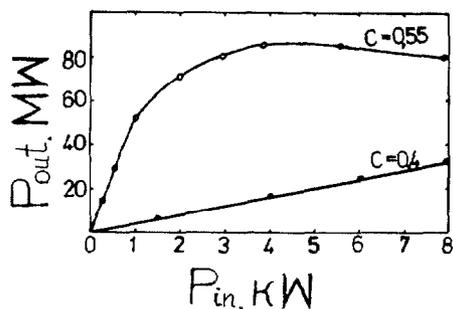
Fig.2. Output power as a function of input signal.
