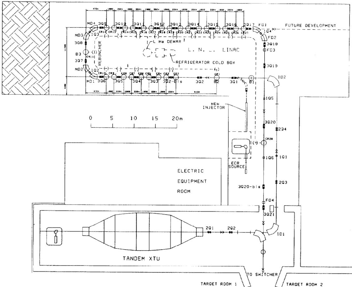
Fig. 1. - Lay-out of the ALPI Linac.
