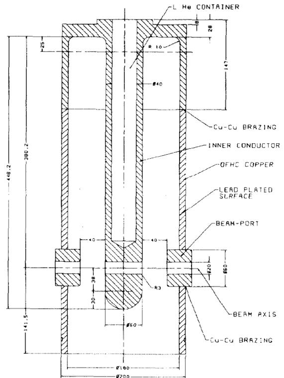
Fig. 2. - Cross section of the quarter wave resonator. [7]
