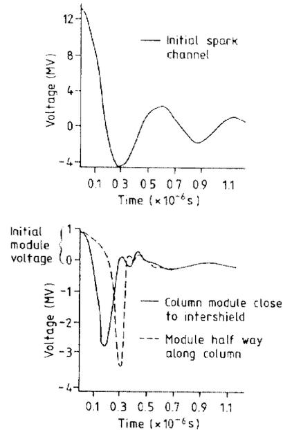
Fig. 7. Calculated transient waveforms for an intershield to tank spark in the Daresbury Tandem.
