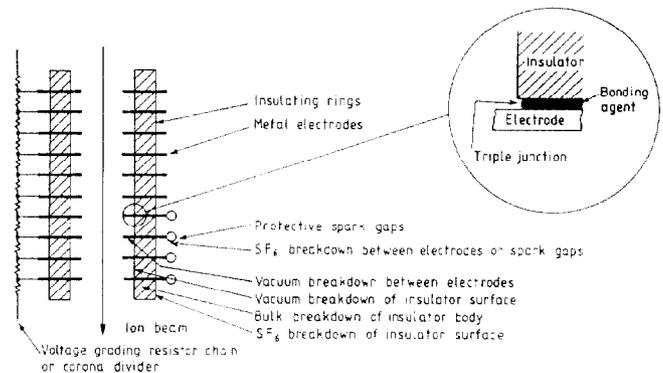
Fig. 4. Various accelerator tube breakdown possibilities.
