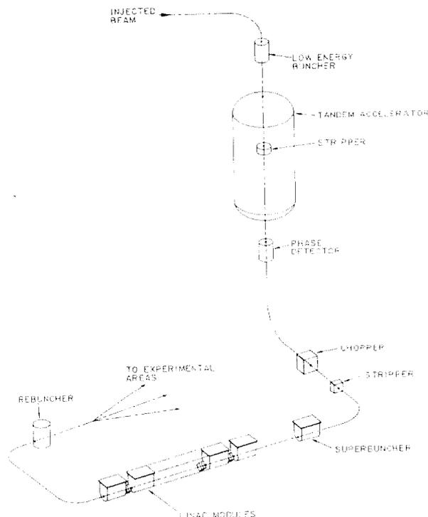
Fig. 9. A generalised layout of a tandem plus booster linac system.
