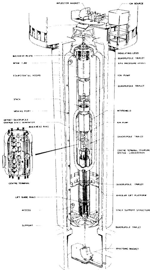
Fig. 2. The Daresbury Laboratory Tandem.
