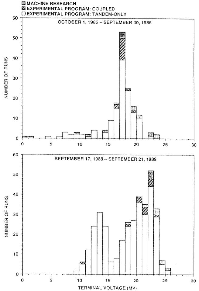
Fig. 6. The voltage performance of the Oak Ridge Tandem before and after installation of the compressed geometry tubes.
