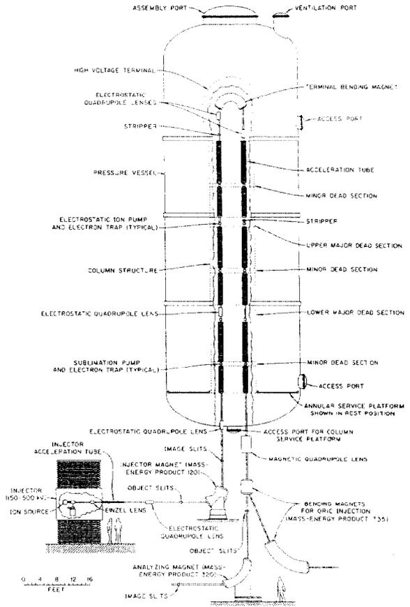
A schematic view of the 25-MV tandem accelerator system
