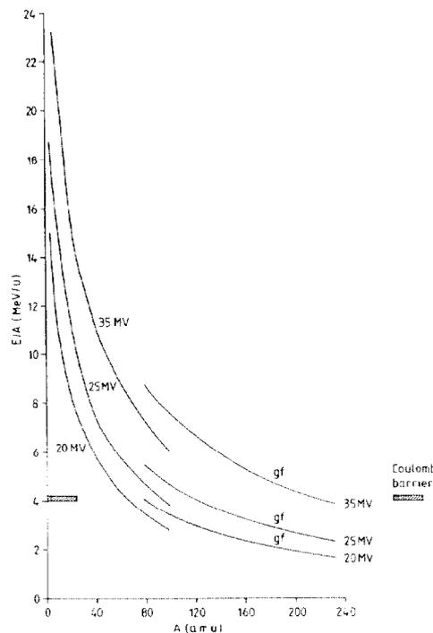
Fig. 1. The output beam energy from tandem accelerators operating at 20 MV, 25 MV and 35 MV. Use of a terminal gas stripper and a second foil stripper has been assumed for  $A > 80$ .
