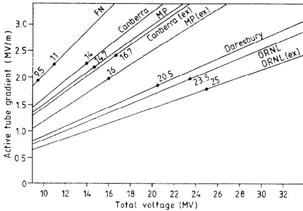
Fig. 5. A summary of active accelerator tube gradients.
