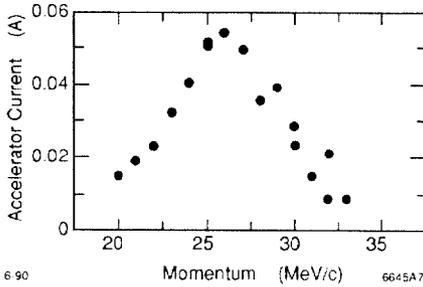
Figure 2: Energy spectrum of two-stage accelerated beam.
