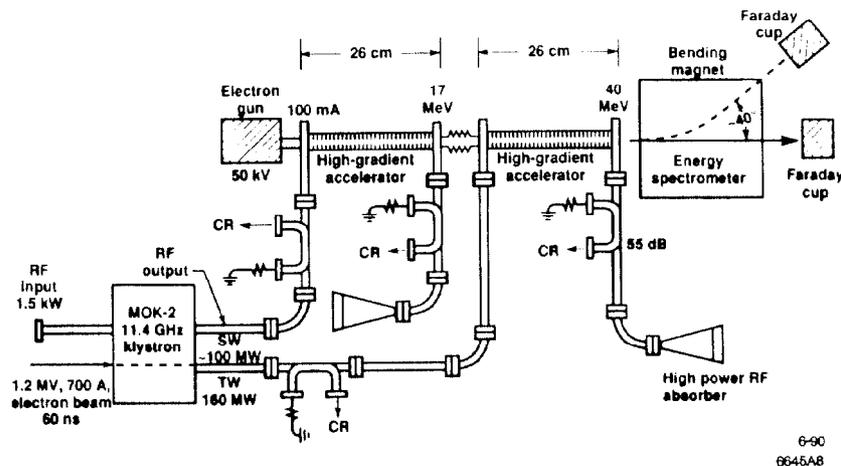
Figure 1: High gradient two-stage accelerator test.
