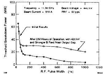
Figure 5: Measured threshold breakdown power vs. RF pulse width for klystron.
