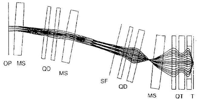
Fig. 3: Final focus system at the Target area for intense beam experiments (OP - takeover point; MS - magnetic sector; SF - stripper point; QD - quadrupole doublet; QT - quadrupole triplet; T - target).
