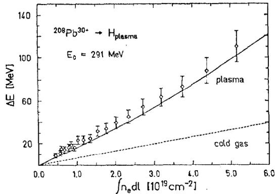
Fig. 8: Energy loss of Pb ions as a function of the free electron density. The dashed line represents the energy loss derived from data tables [22].
