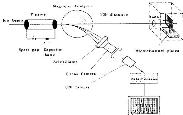
Fig. 6: Set up of the beam plasma interaction experiment with a z-pinch plasma. Time of flight technique is applied to measure the energy loss in the plasma, and a detector system with magnetic analyzer serves for charge state analysis of the ion beam.
