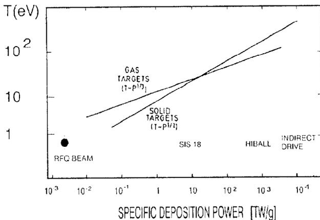
Fig. 2: Matter temperatures of ion beam heated plasmas as a function of specific deposition power [7]. The first experimental result of ion beam heated plasmas with the intense beam from the RFQ accelerator is shown. The plasma temperature was just below 1 eV.
