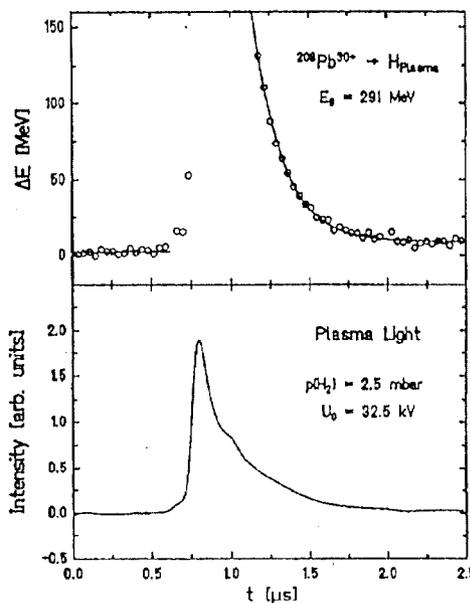
Fig. 7: Energy loss of Pb ions in a dense hydrogen z-pinch plasma (upper part), and the plasma light output signal from the z-pinch measured along the pinch axis.
