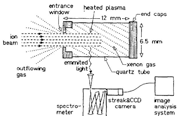
Fig. 4: Set-up of the intense beam experiment at the RFQ accelerator. A closed gas target is heated with an intense ion beam.
