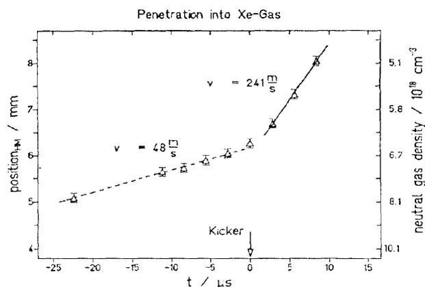
Fig. 5: Penetration velocity of a high and a low intensity beam into a Xe gas target.
