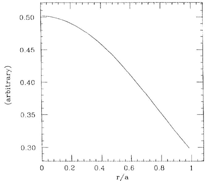
Both the plasma and dielectric pipe exhibit similar problems. In the plasma even a uniform distribution in the drive bunch gives rise to transverse forces seen by the trailing bunch. In the dielectric an offset beam from the center of the pipe is necessary to excite the transverse forces.
