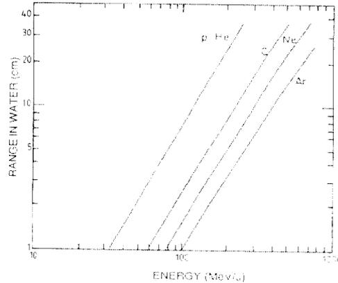
Fig 1 : Range of ions in water as a function of kinetic energy
