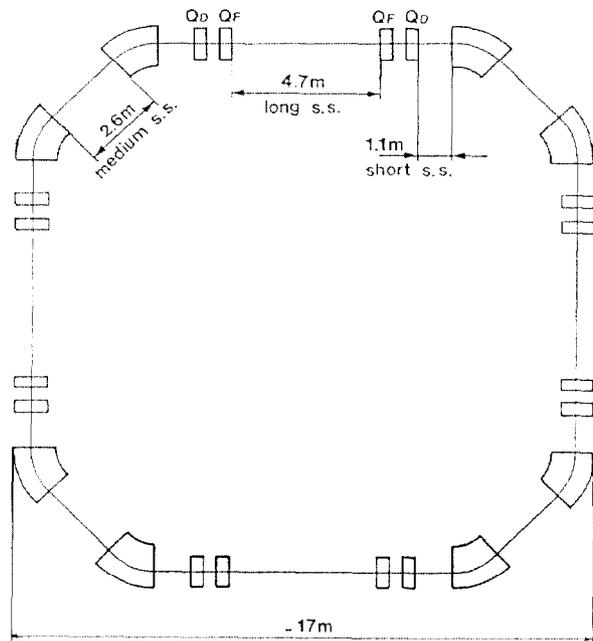
Fig 12 : An arrangement of EULIMA synchrotron lattice
