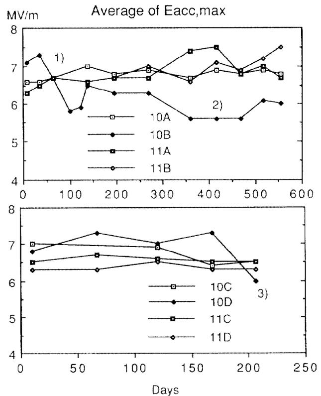
Fig. 3 Change of the maximum accelerating gradient in the ring.
