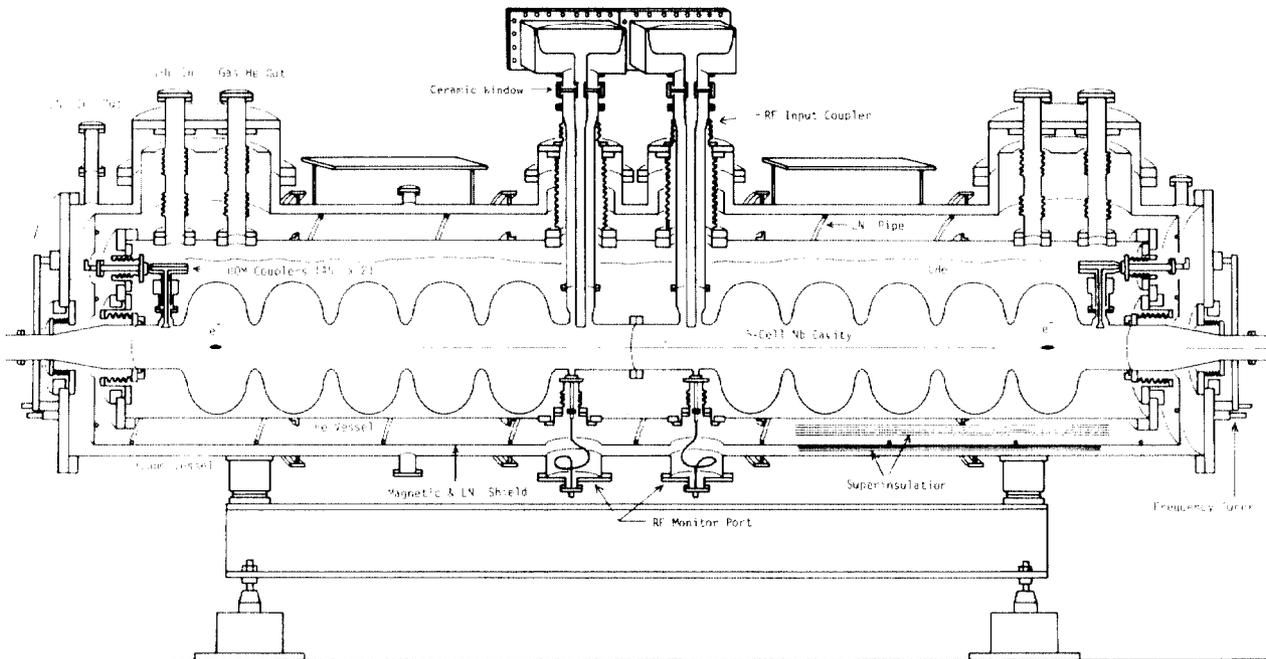
Fig. 2 TRISTAN superconducting cavities in a cryostat.
