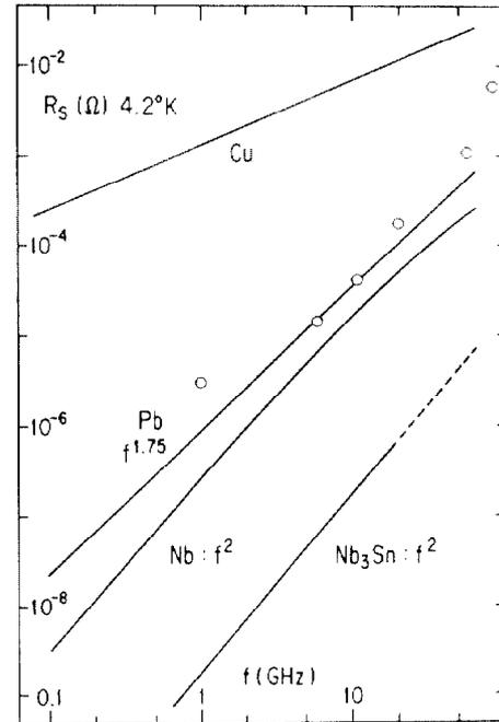
Fig. 1  $R_{BCS}$  of well investigated superconductors,  $\circ$ : the best values of YBa<sub>2</sub>Cu<sub>3</sub>O<sub>7-x</sub>.
