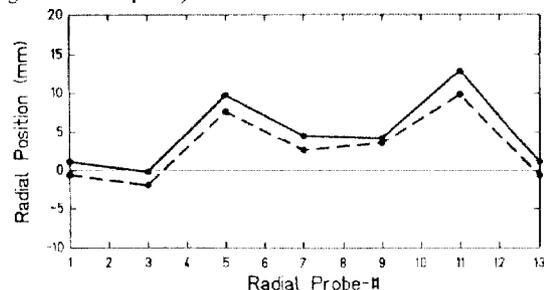
Fig. 1: Closed orbit at 11.4 MeV/u measured at six out of twelve positions. Solid line: preceding virtual accelerator operated at 11.4 MeV/u; dashed line: preceding virtual accelerator ramped to 200 MeV/u
