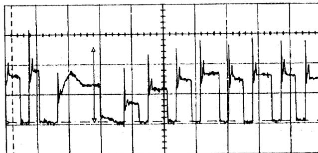
Fig. 5: Supercycle operation in SIS - seven cycles accelerating up to 100 MeV/u, every eighth cycle up to 1700 MeV/u. (2 s/div.)
