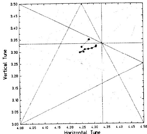
Fig. 2: Measured tune (solid line) and set values (dashed line) during acceleration from 11.4 to 150 MeV/u and changing of the focusing from triplet to doublet.
