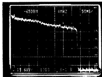
Fig. 4: Narrow-band signal of a 1000 MeV/u  $\text{U}^{22+}$  bunched beam on the flat top (50 ms/div.)
