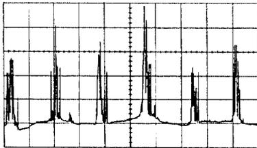
Fig. 6: 300 Hz spill modulation observed during the first tests of resonance extraction (2 ms/div.)
