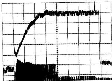
Fig. 3: Accelerating  $\text{Ar}^{19+}$  up to 1000 MeV/u. upper trace: absolute particle current, not normalized to  $\beta$ . lower trace: RF voltage during acceleration (200ms/div)
