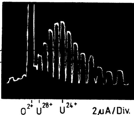
Fig. 3: Uranium from the 14 GHz ECR source
