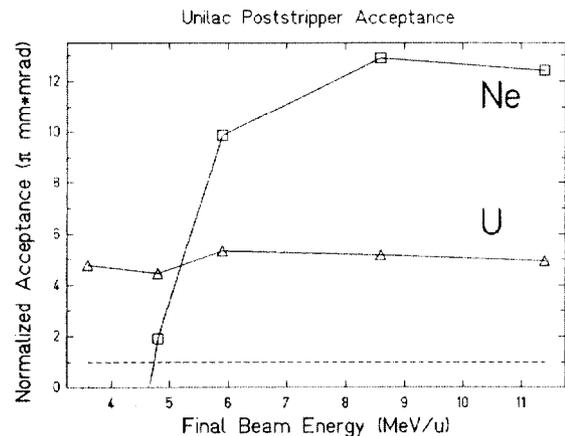
Fig. 5: Calculated overall acceptance of the UNILAC poststripper section for simultaneous acceleration of  $\text{Ne}^{6+}$  and  $\text{U}^{28+}$  to various energies in "ion switching" mode. The dashed line indicates the maximum beam emittance.
