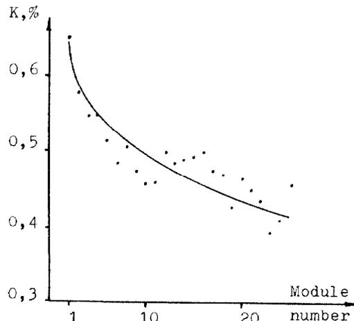
Fig.2. The coupling coefficient between the tanks and the bridges against the module number.
