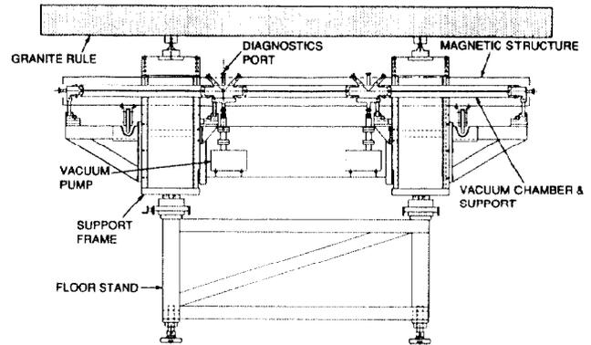
Fig. 5 Side view of the Darmstadt undulator (courtesy of Spectra Technology Inc.)
