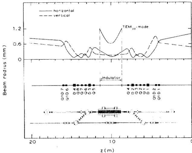
Fig. 4 The FEL bypass and the beam envelopes calculated by TRANSPORT
