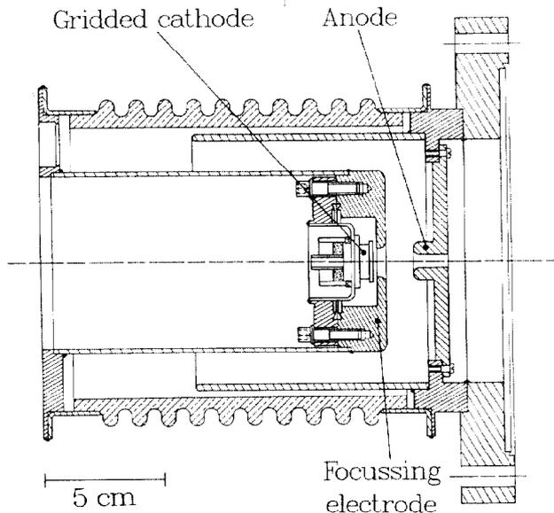
Fig. 3 Mechanical layout of the high current electron gun
