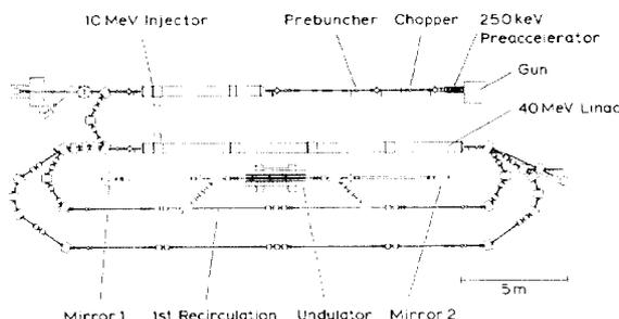
Fig. 1 The 130 MeV accelerator and the FEL experiment
