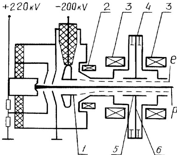
Fig. 4. The electron-ion injector and the electron buncher of the second version of linac.
