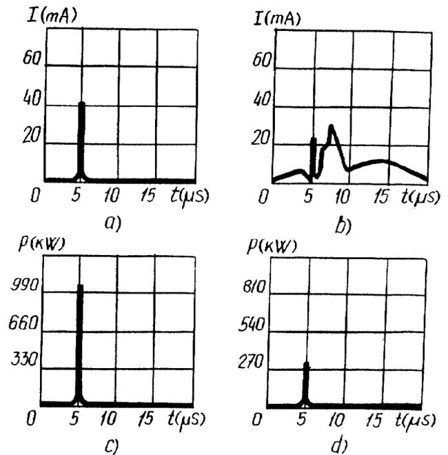
Fig. 5. The signals oscillograms showing (a) accelerated protons current on the Faraday cup screened by foil, (b) proton current on the foil, (c) accelerating resonator RF power pulse, (d) the electron buncher RF power pulse.
