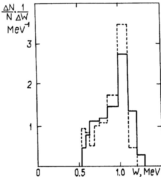
Fig. 3. Energy distribution of protons accelerated in the first version of linac with electron beam excitation (solid) and with only external RF power supply (dashed).
