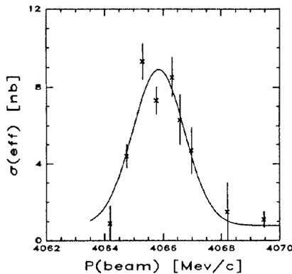
Figure 2: The  $J/\psi$  resonance was observed by the E-760 experiment while scanning the beam. These data are not fully corrected and should not be taken to be definitive.
