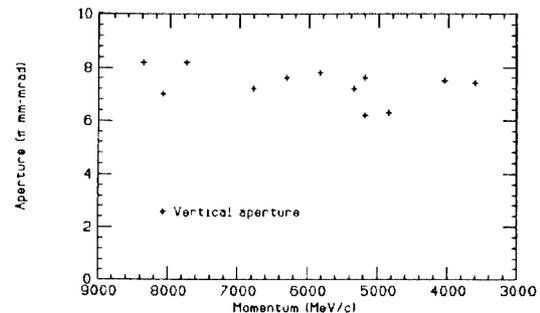
Figure 1: The vertical aperture is shown as a function of momentum. The horizontal aperture is similar except for a reduction in aperture just below the energy crossing.
