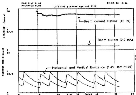
Figure 3: The on-line monitoring display of beam lifetime and emittance is shown. Oscillations in the horizontal and vertical emittance were observed with the transverse dampers set to the wrong phase.
