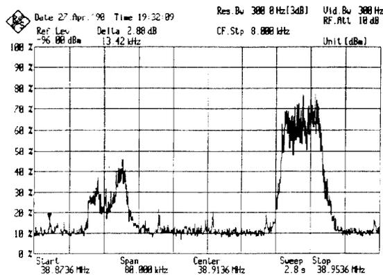
Fig.6: Schottky spectrum with deuteron peak (left) and oxygen peak (right)
