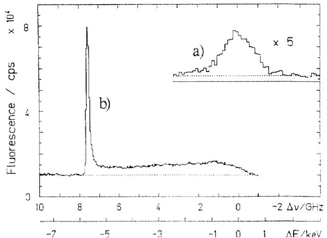
Fig.7: Laser fluorescence signals; a) shows the initial and b) the "compressed" velocity distribution.
