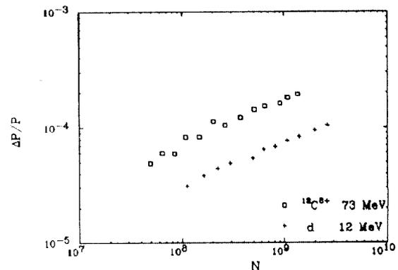
Fig.2: Measurement of momentum spread as a function of particle number for deuterons and carbon ions stored with electron cooling under the same experimental conditions
