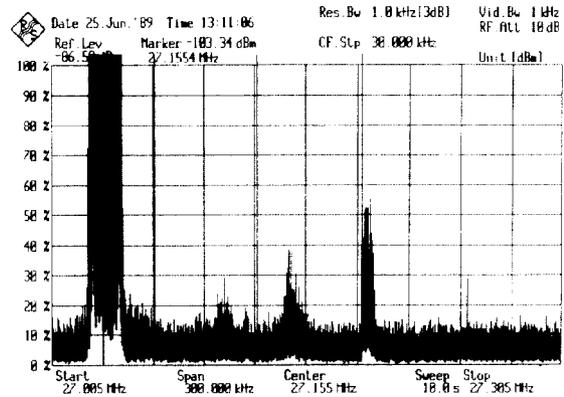
Fig.5: Schottky spectrum during multiturn injection with electron cooling to increase the intensity of the accumulated beam
