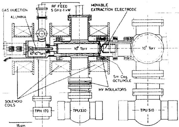
Fig. 1 Schematic view of the ion source
