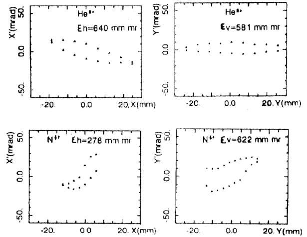
Fig. 6 Horizontal (left) and transverse (right) emittances respectively for a 27  $\mu\text{A}$   $\text{He}^{2+}$  (top) and a 10  $\mu\text{A}$   $N^{4+}$  beam (bottom)
