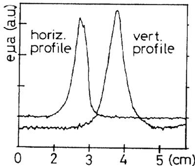
Fig. 5 Horizontal and vertical profiles for a 10  $\mu\text{A}$ ,  $N^{4+}$  beam, at the image slit
