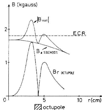
Fig. 2 Magnetic field distribution as a function of the radius at the centre of the II stage
