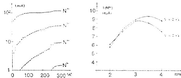
Fig. 4 Dependence of the ion current from microwave power and source to puller distance
