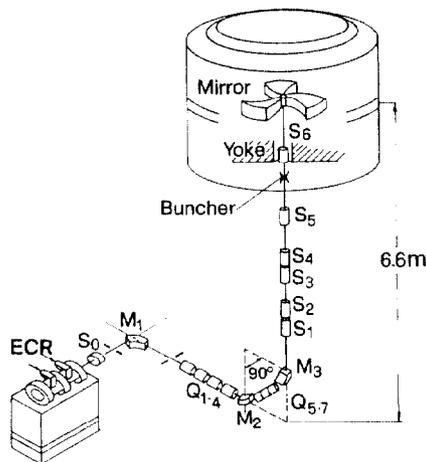
Fig. 3 View of the axial injection system
