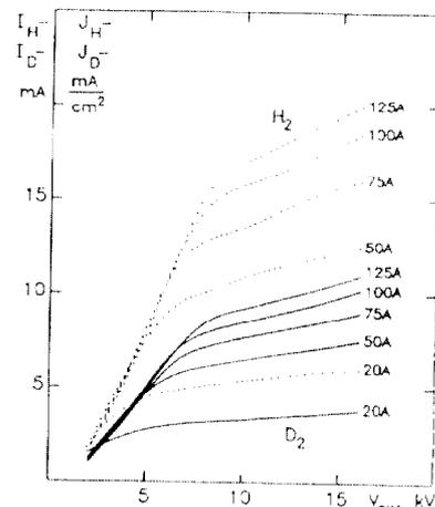
Fig. 1: Negative ion field vs the extraction voltage  $V_{ex}$ , with arc current as parameter, for hydrogen (dotted) and deuterium (solid lines).
