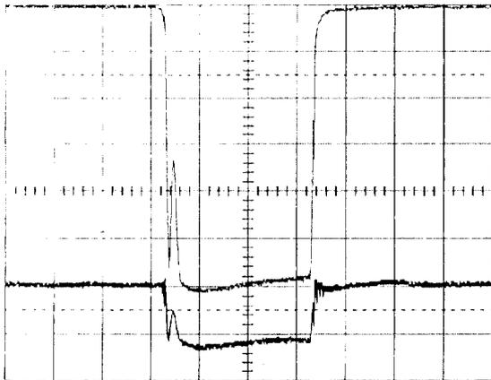
Fig. 6:  $H^-$  current (upper trace, 5 mA/div.) and total extractor supply load (lower trace, 50 mA/div.). Time Scale = 0.5  $\mu$ s/div. Taken with cesium in the source.
