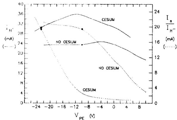
Fig. 5:  $H^-$  current and electron-to- $H^-$  ratio, as a function of the plasma electrode bias, with and without cesium.  $I_{arc} = 150$  A,  $V_{arc} = 250$  V,  $V_{ext} = 16$  kV. The dots indicate the floating potential.
