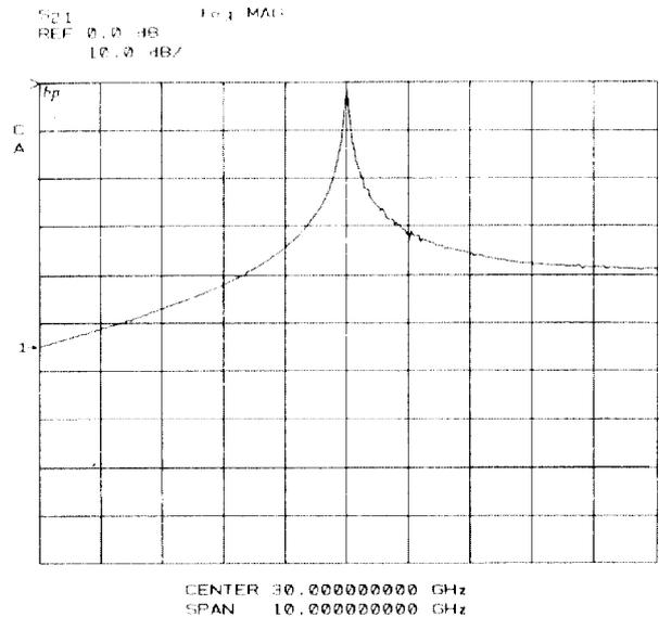
Fig. 4 30 GHz waveguide filter response
