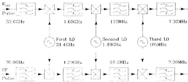
Fig. 2 Receiver configuration for 33 GHz position pick-up cavity
