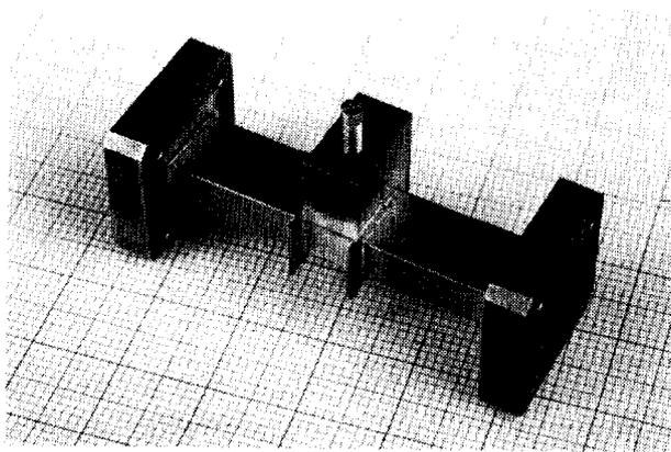
Fig. 3 30 GHz waveguide filter
